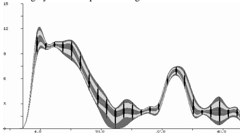
**Figure 2** A fuzzy B-spline fitting a set of 1D data: B-splines "shells" at different presumption levels are shown in different gray tones; the black vertical bars are a pictorial representation of the fuzzy constrains taken into account by the fitting algorithm.
